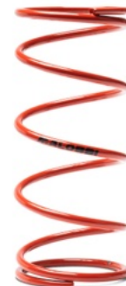
External Ø 67.2 x 130 mm Ø Wire 5 mm - K 6.2
