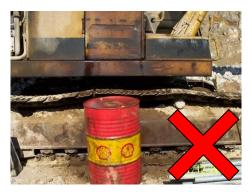
(viii) Place the machinery on a paved area to avoid oil leakage or spillage on ground when carrying out the maintenance work.
