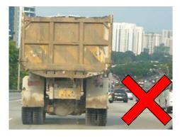
(vi) Cover the load on vehicles entirely by clean impervious sheeting or mechanical cover.
