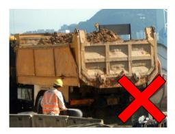
(iv) Cover the load on vehicles entirely by clean impervious sheeting or mechanical cover.
