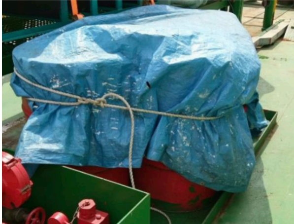
Providing proper drip tray for chemical storage to prevent accidental spillage
