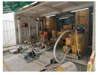
Carrying out de-bagging, batching and mixing processes for production of concrete using bagged cement in an area sheltered on the top and the 3 sides.
