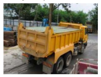
Covering dusty materials on dump truck entirely by impervious sheeting to avoid dust emission during transportation.
