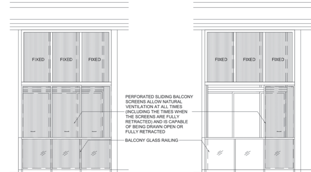
#44-01, #44-02, #44-04, #44-06, #44-08, #44-09, #44-10, #44-11, #44-12: TYPICAL RETRACTABLE BALCONY SCREEN (CLOSED) - ELEVATION 1
